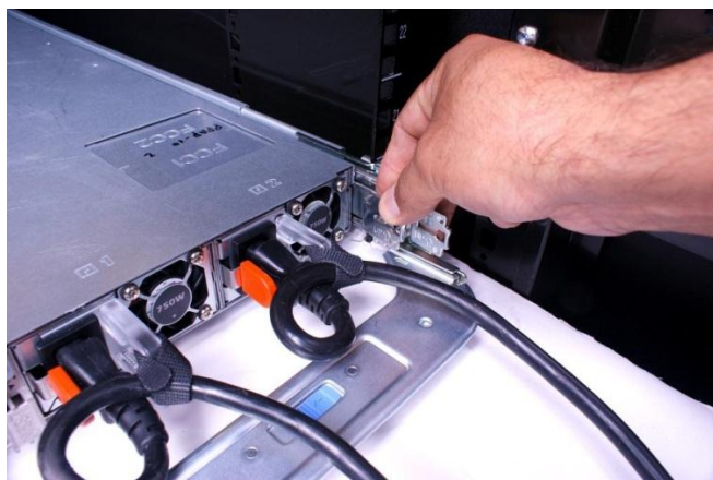
Figure 3. Attaching the inner CMA attachment bracket
